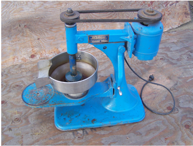
Western Machinery Lab Flotation Cell. Driven by .25 HP Motor.
