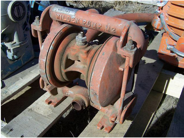
Used Wilden Diaphragm Pump. 1 in. x 1.5 in. Model M-2.
