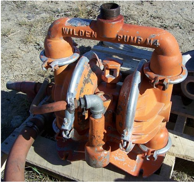
Used Wilden Diaphragm Pump. 1.25 in. x 1.5 in. Model: M-4
