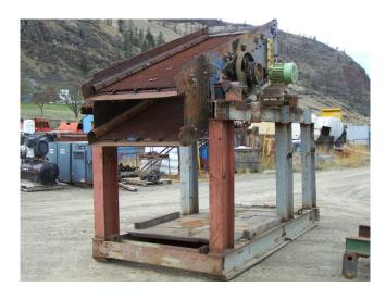
Used Tyler Screen. 4 ft. x 8 ft - 2 Deck Inclined Screen. Mounted on skid frame. Can be supplied with discharge conveyor.
