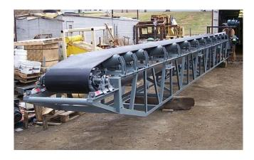
Used Truss Conveyor. 24 in. x 45 ft. Long. Steel tail; steel head pulley. Right angle reducer and motor. SUPPLIED RECONDITIONED.
