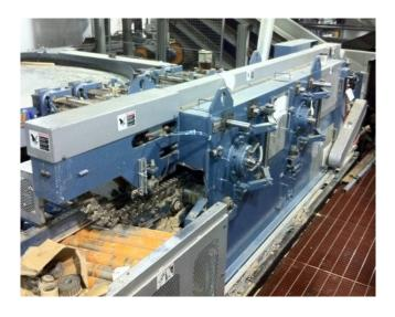
Used Tronco 2 in. x 12 in. 4 Saw Edger. 300 ft. per Minute Feed Rate. 2 - 30 HP Arbor Drives.
