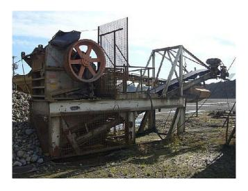
Used Telsmith Jaw Crusher. 15 in. x 38 in. 60 HP Motor & 36 in. Discharge Conveyor. All Mounted on Common Frame.
