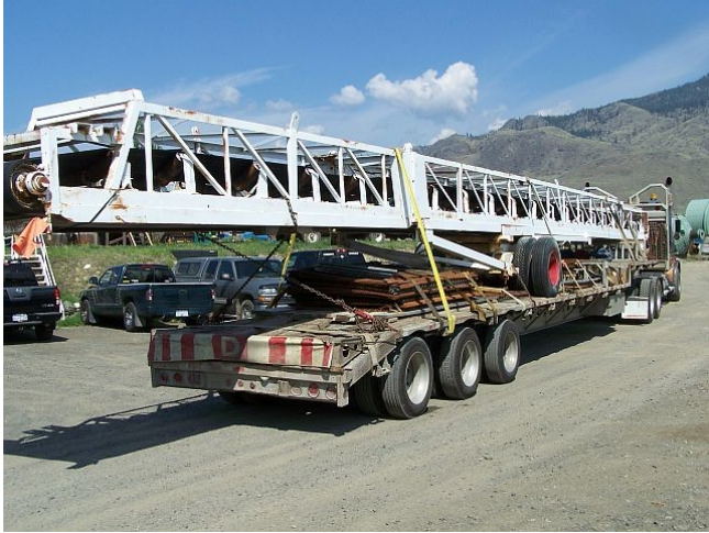
Used Stacking Conveyor. 36 in. x 70 ft. Long. Folding Truss Frame for Transport.
