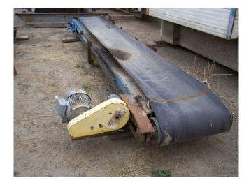
Used Square Tubing Conveyor. 24 in. x 15 ft. Long. 5 HP Motor through Radicon Reducer.
