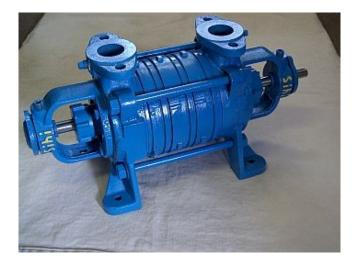
Used SIHI Centrifugal Pump. 1.5 in. x 1.5 in. CAO Series. Three Stage Self Priming.
