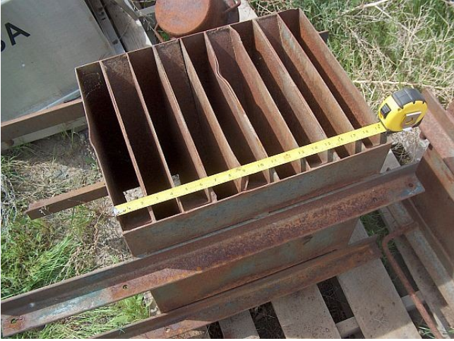
Used Sampler. 9 Slot, 2 in. Sample Splitter.
