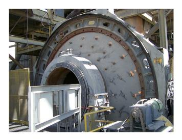
Used Sag Mill. 20 ft. x 7 ft. Long. 800 HP. Steel Lined. Inching Drive.
