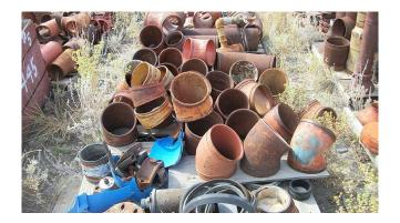
Used Pipe Fittings. 8 in. to 12 in. Grooved Fittings, Clamps, Elbows, Ts, Ys & Reducers.
