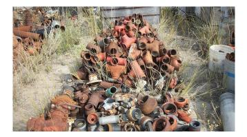
Used Pipe Fittings. 1 in. to 3 in. Grooved Fittings, Clamps, Elbows, Ts, Ys & Reducers.
