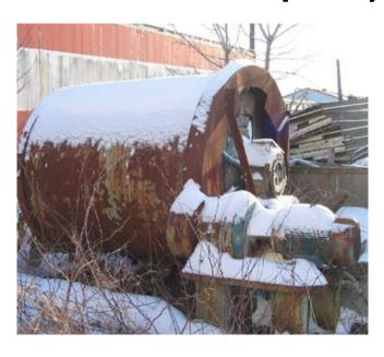
Used Patterson Ball Mill. 56 in. dia. x 72 in. Long. Ceramic Lined Batch Mills. Electric Motor Drive.
