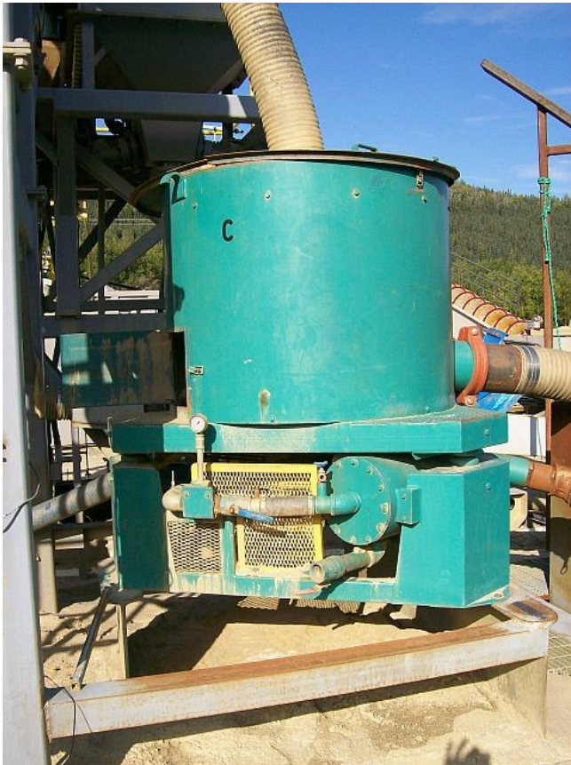
Used Knelson Concentrators. 30 in. Supplied with Poly G5 Cone.
