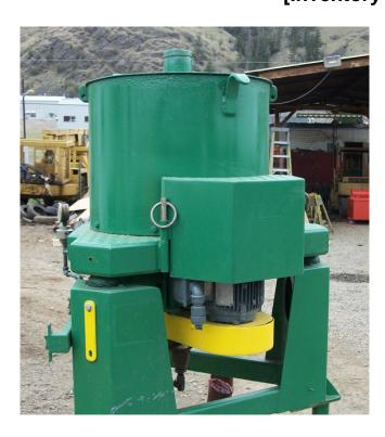
Used Knelson Concentrator. 12 in. Supplied with Poly Bowl. Driven by 2 HP Motor. Unit is in Exellent Condition!
