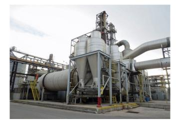
Used ICM Stainless Steel Rotary Dryers. 13.5 ft. dia. x 40 ft. Long. Model: 40136L. Eclipse 22V Burner with 400 HP Fan. Each System has 4 - 8 ft. dia. Cyclones.
