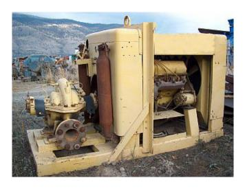
Used High Pressure Water Pump. 5 in. x 4 in. Ford V8 Gas Engine.
