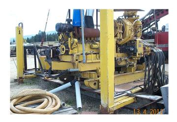
Used HD 900 Marooka Diamond Drill. HD 900 PQ Head. Dump Mast. American Mud Pump. Drill is Recently Serviced.
