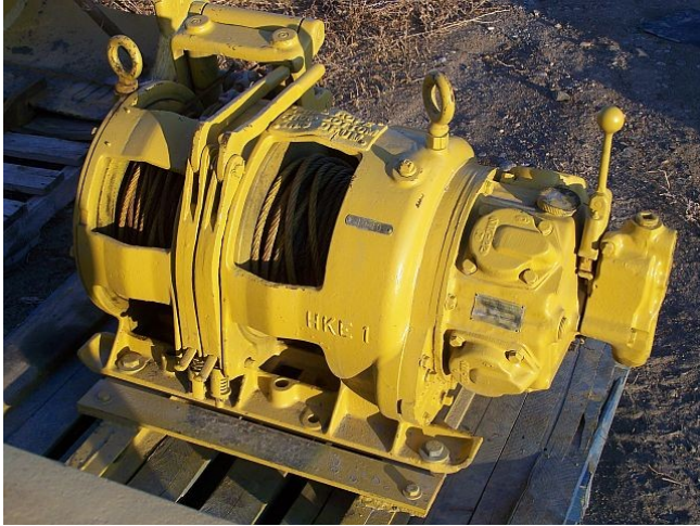
Used Gardner Denver (Slusher) Hoist. Model: HKE. Double Drum - Air Operated.
