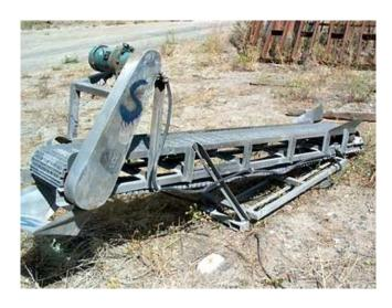
Used Food Product Conveyor. 12 in. wide x 9.5 ft long. Stainless Steel Construction with Perforated Poly Hinged Belt, 1/2 HP Chain Drive
