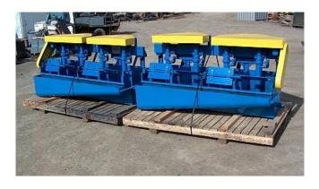
Used Floatation Cells. Bank of 6 #8s. Comes with paddle shaft and drive motors. Unit refurbished, 2 extra cells added and converted to 2 banks of 4.
