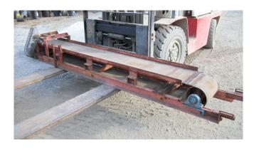
Used Flat Belt Conveyor. 14 in. x 9.5 ft. Long 8 in. Head and Tail Pulley.
