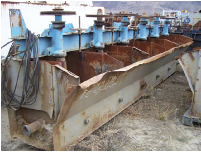
Used Denver Flot Cells. Bank of 6. Sub A #18 Specials.
