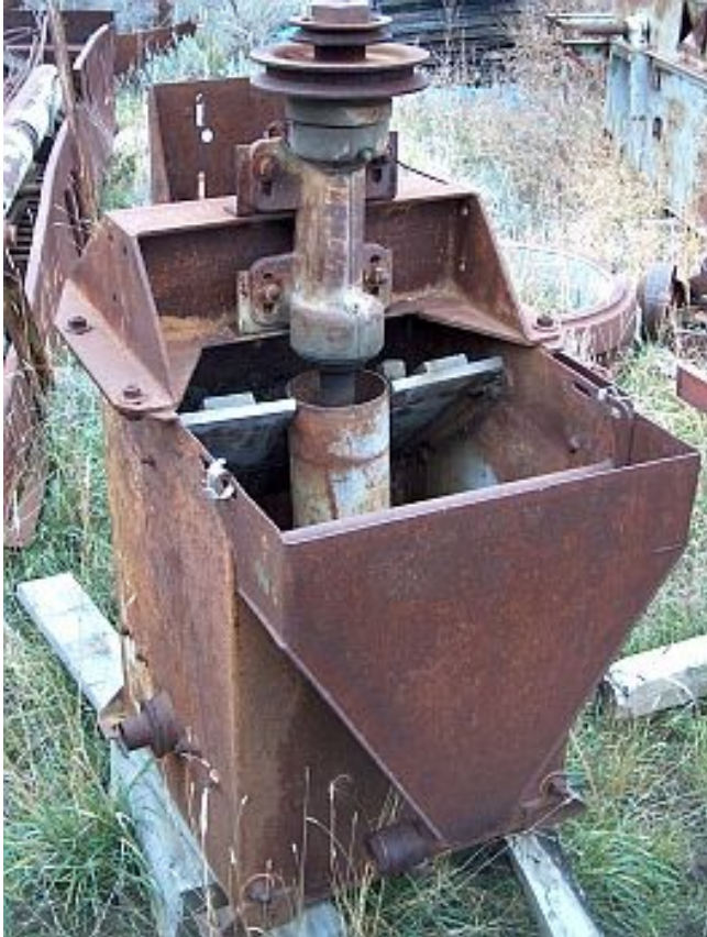
Used Denver #15 Sub A Single Flot Cell. Supplied with Discharge Launder.
