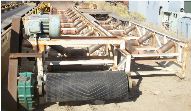
Used Channel Conveyor. 36 in. x 80 ft. Long. 15 HP Motor.
