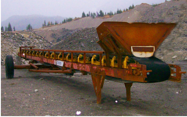
Used Channel Conveyor. 18 in. x 45 ft. Long
