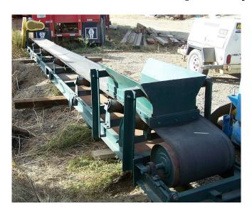
Used Channel Conveyor. 18 in. x 30 ft. Long. 2 HP Single Phase Electric Motor.
