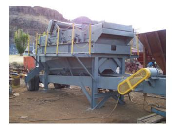
Used Cedar Rapids Horizontal Portable Screen. 5 ft. x 16 ft. 2 Deck On Single Axle Chassis with Product Chutes and 30 in. Discharge Belt.
