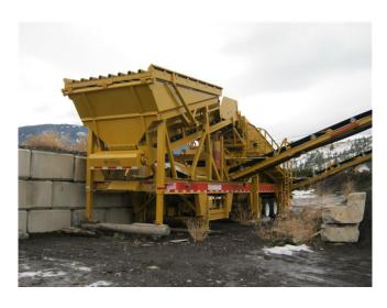
Used CEC Portable Screen. 6 ft. x 16 ft. - 3 Deck. Incline Style. Diesel Driven with Deutz Engine, 200 HRS.
