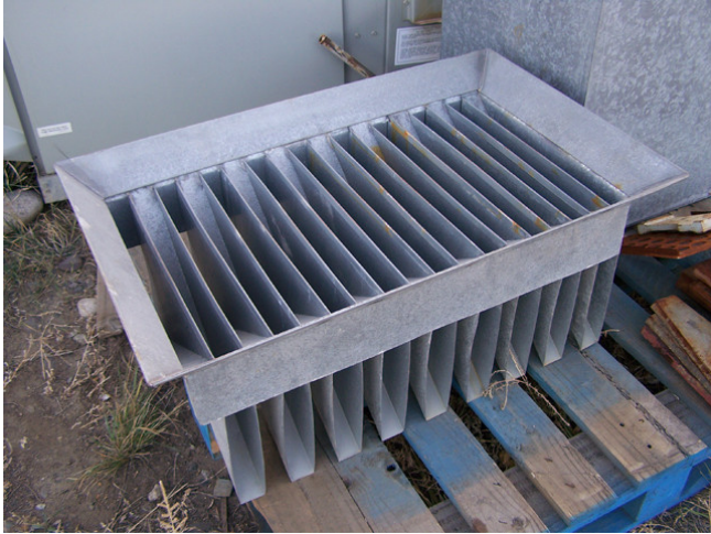
Used Assay & Lab Equipment. Sample Splitter 13 - 8 in. Openings, 18in. Chute, 28 in. x 16 in. Feed
