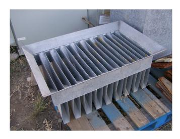
Used Assay & Lab Equipment. Sample Splitter 13 - 8 in. Openings, 18in. Chute, 28 in. x 16 in. Feed
