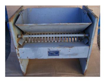
Used Assay & Lab Equipment. Gilson Model SP-2. Adjustable Splitter With Leaver Release Hopper.
