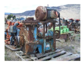
Used Allis Chalmers Slurry Pumps. 5 x 4 x 14 SRLC. Supplied with Overhead Motor Base. Can be Supplied with or without Motor. As is or refurbished.
