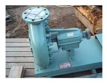
Used Allis Chalmers Centrifugal Pump. Model: F4D1-391. Supplied with Cast Iron Housing and 13 in. Stainless Steel Impeller.
