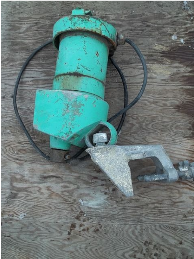
Used Agitators. Lightnin Mixer. Single Phase. 1/3 HP.
