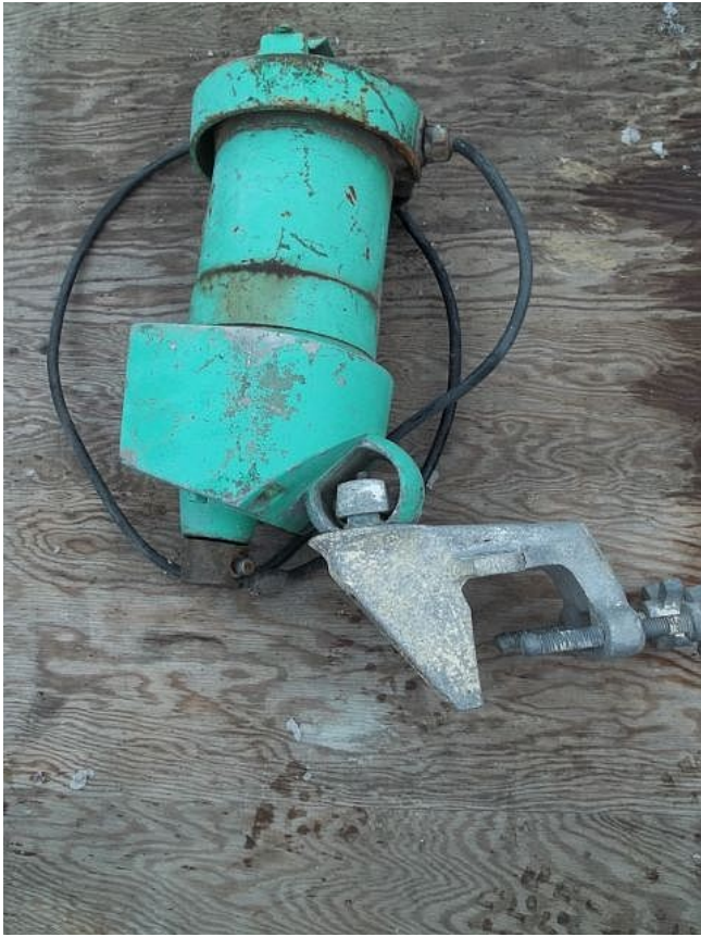
Used Agitators. Lightnin Mixer. Single Phase. 1/3 HP.
