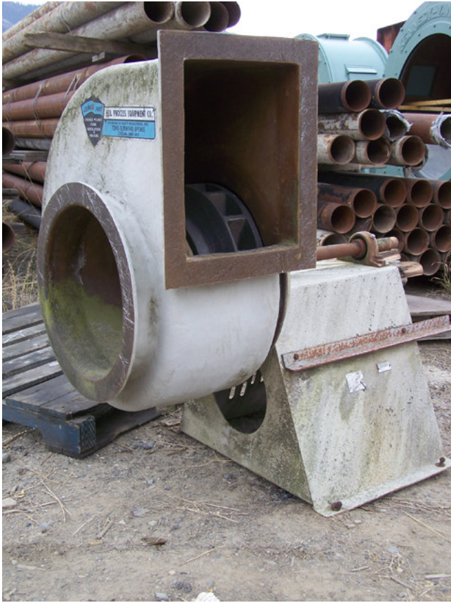
Heil Process Equipment Fibreglass Blower. S/N 842232.
