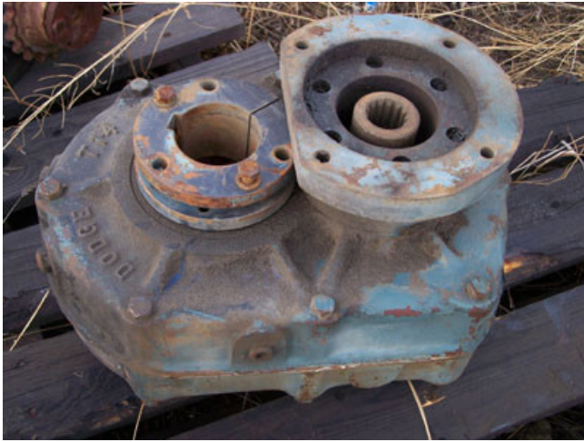
Shaft Mount Speed Reducer - Dodge, TXT 4, 5:1, Spline Drive
