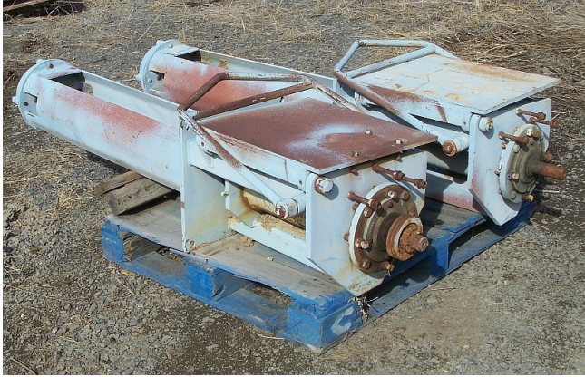
Sala Sump Pumps. 1 inch. Model: VASA-G-120-161. 5 HP electric motor.
