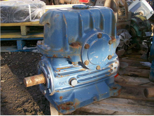
Renolds Size 5 Right Angle Reducer. 29:1 Ratio.
