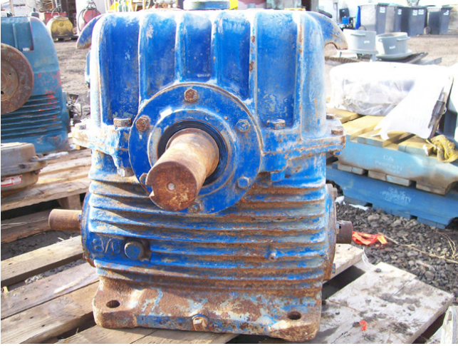
Renold Size 8 Right Angle Reducer. 18:1 Ratio.
