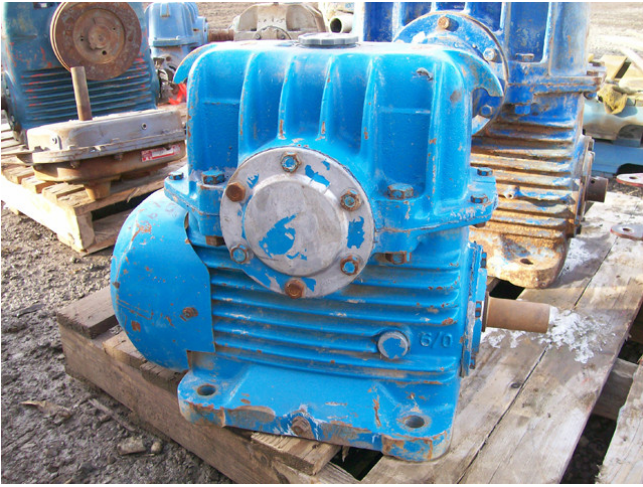
Renold Size 6 Right Angle Reducer. 40:1 Ratio.
