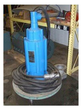
Reliance 50hp, 575 volt Submersible Aerator Pumps. Rebuilt complete with 75ft of cable.
