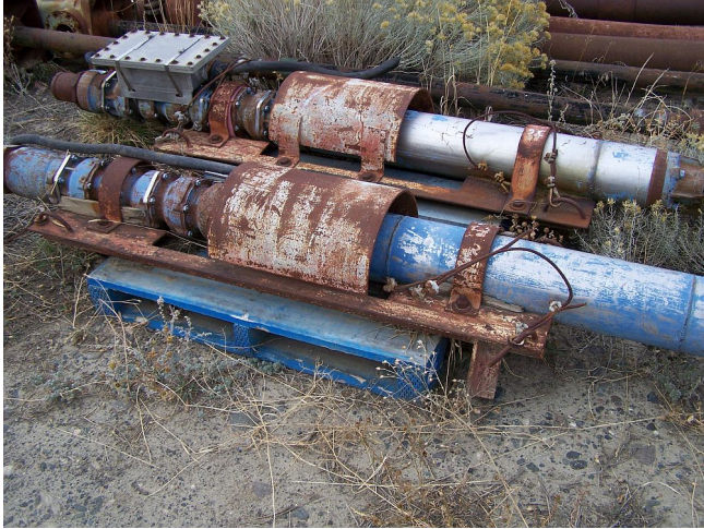
Pleuger 60 Hp Deep Well Submersible Pump. 6 Stage, 575 Volt. Model P82-6.
