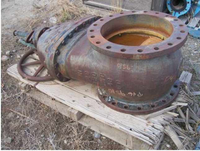
MH 20 in. Gate Valve. 150 PSI.
