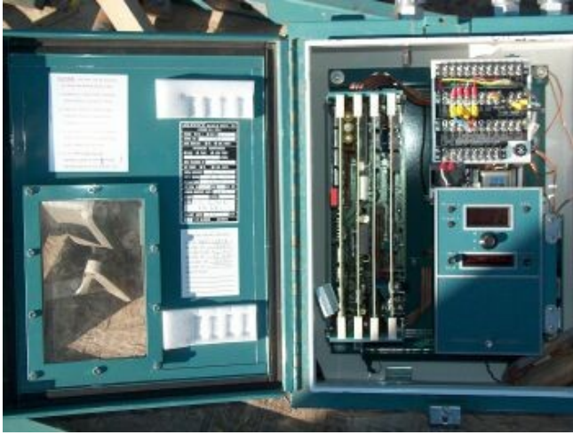
Merrick belt scale. For 18 in. conveyor.
