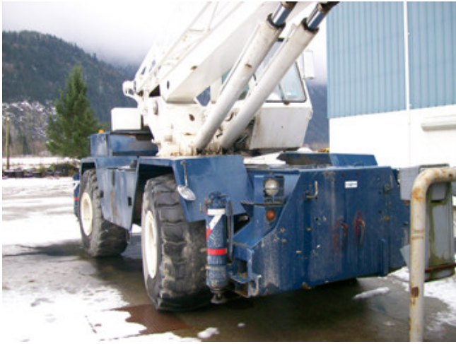
Lorain / Koehring LRT 330 Mobile Crane. 81 FT Boom.
