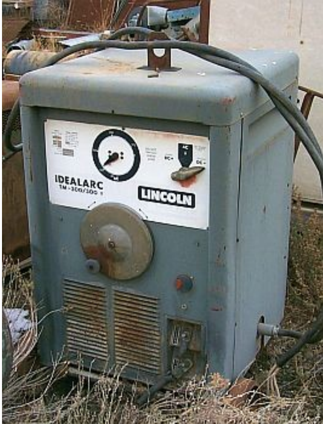
Lincoln 300 Amp AC/DC Electric Welder. Model TM-300/300. 575 Volt Single Phase.
