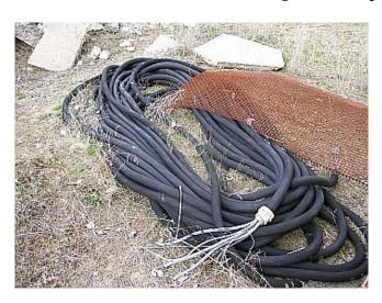
Length of cab tire. 350-feet by 2-inch diameter.
