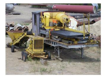
Gold Mining Equipment. Placer/Tailings Pilot Plant. Trommel and Ball Mill, plus Full Size Gold Concentrating Table. All on 35 ft. Highboy Trailer. Complete with feed conveyor and generator
